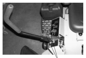
Figure. 11 Lap Bar Mounting Bolt and Nuts
